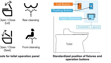
TOTO was influential in the establishment of standardized graphical symbols for toilet operation units (ISO 7000) and standardization of accessible design, including the shape and color of the flushing and call buttons and their arrangement together with the paper
