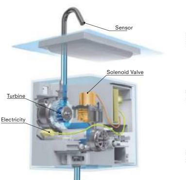
This ECOPOWER touchless faucet uses the flowing water to generate the electricity it needs to operate. There is no need for electrical wiring, making installation and renovation easier
